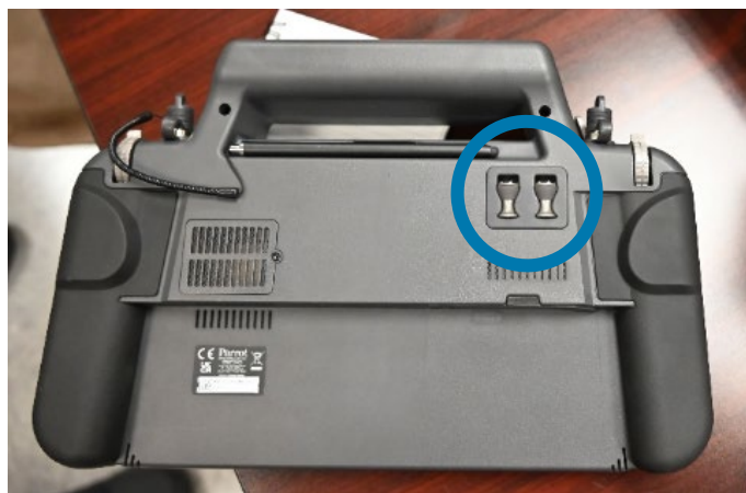
Figure 4-15 Parrot ANAFI USA GOV joysticks (circled) stored on the rear of the GCS
