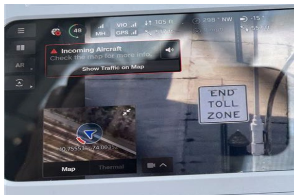
Figure 4-25 Alert of incoming aircraft on the Skydio X10D GCS
