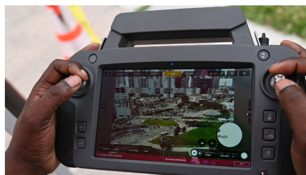
Figure 4-13 Banner interference indicators (yellow and red alerts across the bottom of the GCS) from the Complex Urban (top) and Urban (bottom) Assessments
