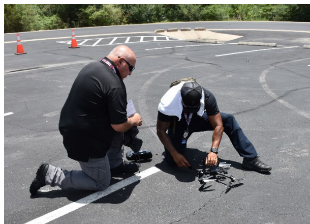
Figure 4-19 Evaluators configuring the and rotors of the Skydio X2D to prepare for takeoff
