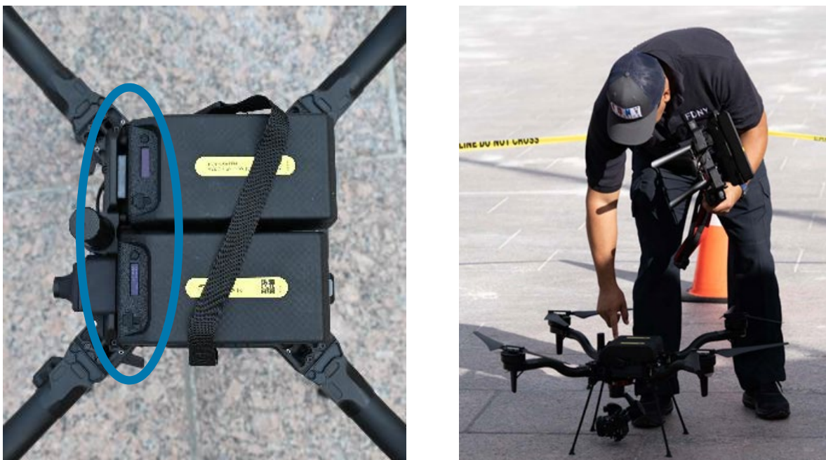
Figure 4-9 Battery placement and power buttons (circled, left) and an evaluator powering on the batteries prior to flight (right)
